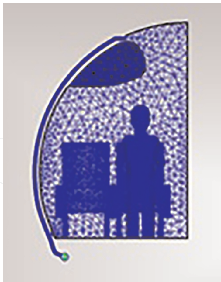
Figure 27. Seated passenger refinement mesh.
